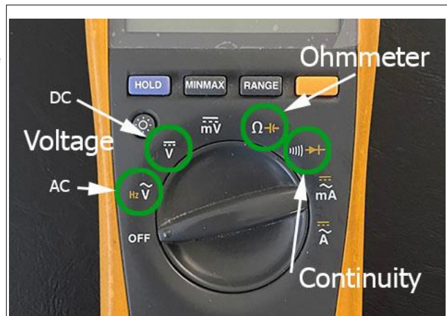
Fig. 1: The main settings used on my Digital Multimeter
