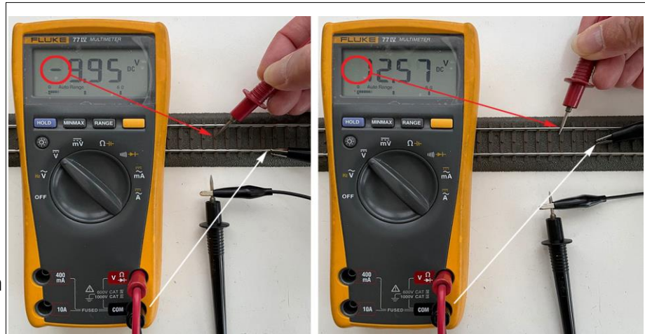
Fig. 2: Using the Voltage DC setting to show polarity.
